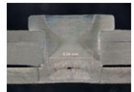
Joint 4 AL 6016 [1.0] - AL 6016 [2.0] - press-hardened steel [1.5]
