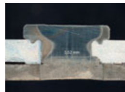
Joint 3 EN AW 7075 [2.0] - press-hardened steel [1.5]
