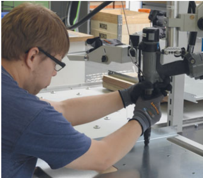
Installation of RIVKLE® blind rivet nuts on thin-walled components for wind energy plants.
