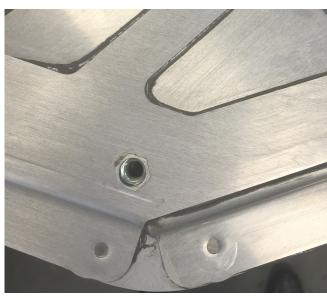
$\mathsf{RIVSET}^{\otimes}$  self-pierce rivets installed in the aluminium body of the Morgan Plus Six
