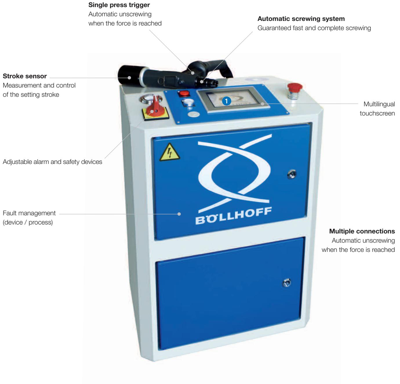
**1** The control unit is equipped with a built-in touch screen that allows the adjustment of the setting parameters, the counters and the alarms and the management of all the sensors.
