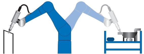
The head can pick fasteners from different bowl feeders (different RIVKLE® fasteners).
