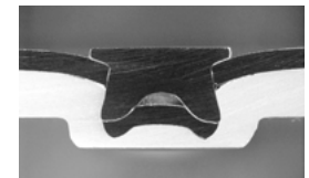
22MnB5, t=1,2 mm Al-Druckguss, t=2,7 mm HDZ 5,5x5 SK H4 Almac
