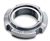
Fine U-Nuts reliably secure shaft bearings, gears and other machine parts against loosening. This is achieved by a plate spring integrated in the nut.
