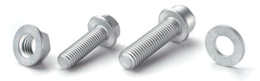
During assembly of the fastener, the radial ribs of the RIPP LOCK® fasteners press into the respective mating surface. The resulting form fit reliably prevents self-loosening of the joint.
