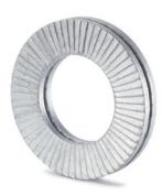
NORD-LOCK® wedge-locking washers are locking elements that comply with DIN 25 201 and which lock the threaded connection by preload force instead of friction.
