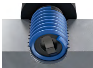
Retraction of the blade and screwing out the installation mandrel
