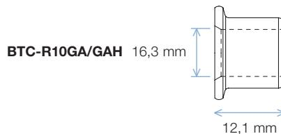
**$d_1$**  = Diameter -  **$l$**  = Length of the stem - = Min. and Max. grip range -  **$\emptyset$**  = Hole diameter -  **$k$**  = Head thickness
