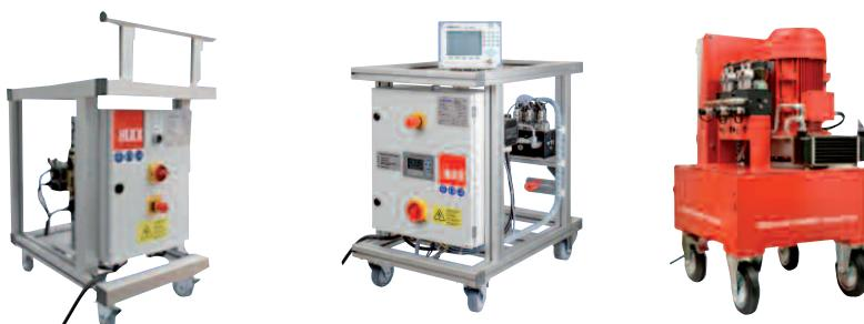
There are 3 options of electrical Powerig™ for a use with hydraulic installation tools.
