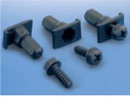
The screw-in blind rivet has been developed for fixing through round holes. To prevent rotation on setting, the surface of the rivet element has an integral flange to lip over the component edge. Other applications are made possible by an underside hexagonal form to the rivet body.
