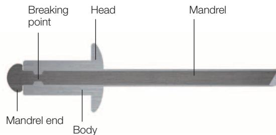
**RIVQUICK® standard rivet after setting**
